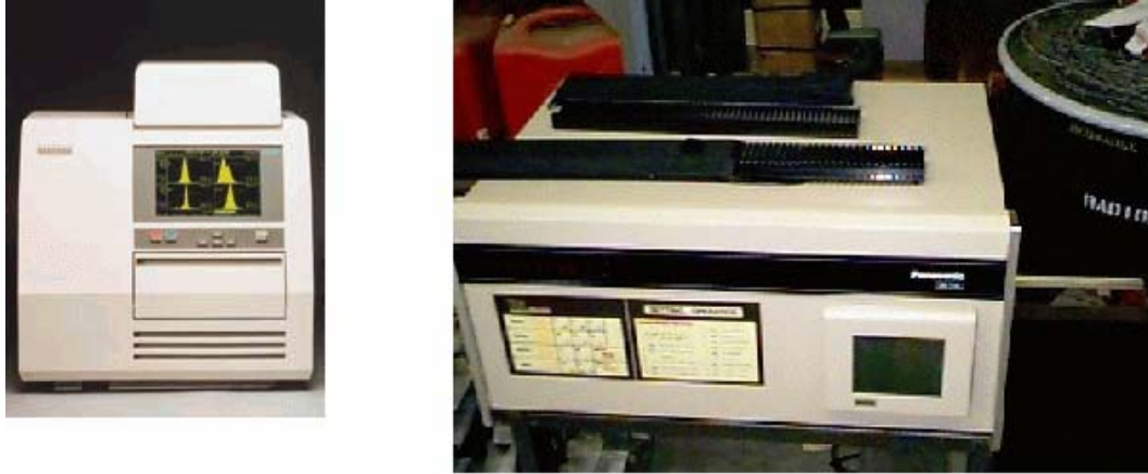
Figure 11: Harshaw and Panasonic TLD readers.
