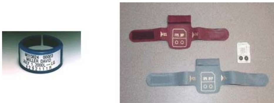
Figure 10: Landauer and NDS extremity TLDs.
