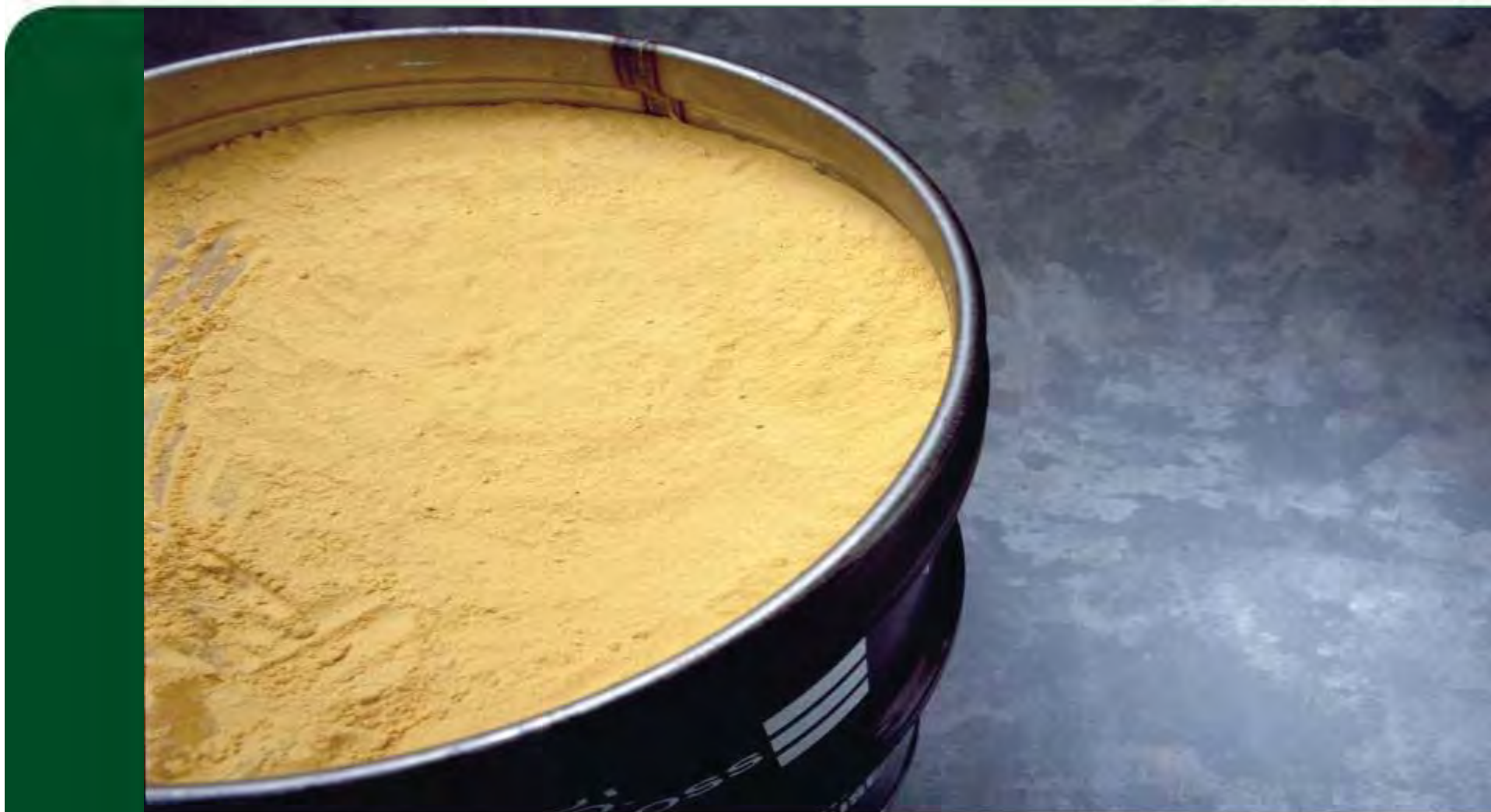
Rabbit Lake Prior to shipping, the yellowcake is packaged into special steel drums.
