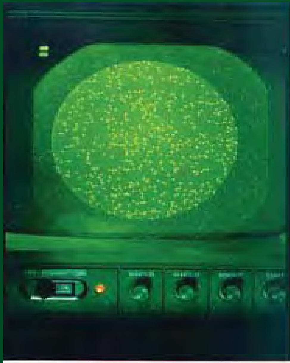
Image of actual radiation impact of radioactive radon progeny Alpha track image from PAD dosimeter National Laboratories, Saskatoon
