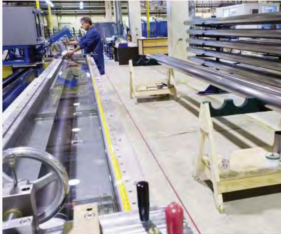
Cameco Fuel Manufacturing Inc. Zirconium tubes are manufactured at the Cobourg facility.
