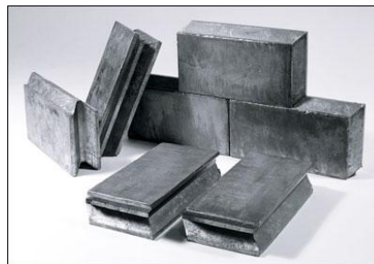
Lead bricks Image courtesy of Radiation Protection Products, Inc.
